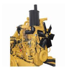
**Cat 3126B Engine.** The Cat 3126B engine is designed for easy maintenance and can be rebuilt for additional service lives. With the HEUI<sup>TM</sup> fuel system, injection pressure is independent of engine speed and provides maximum fuel delivery efficiency with low emissions.
