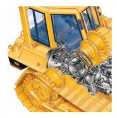
**Torque Converter.** The D5N single-stage torque converter efficiently responds to changing load conditions by providing torque multiplication, therefore increasing drawbar pull. It provides protection to the drive train components by preventing shock loads from heavy dozing applications. The torque converter is efficiently matched to the power train components and provides the superior performance you need.
