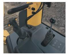
Work Tool Controls. Low effort pilot operated hydraulic controls make the D5N easy to operate and provide sure, precise blade control with less operator fatigue. Ergonomically shaped blade and ripper controls provide increased operator comfort during long shifts.
