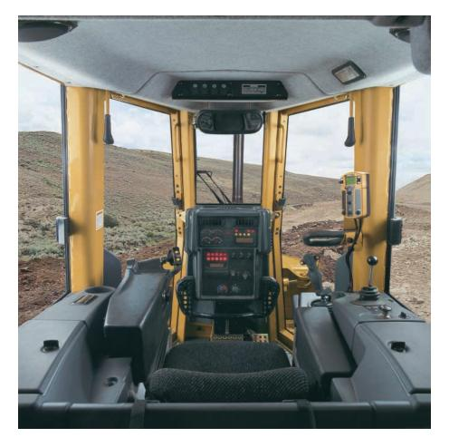
**Cab.** The design is spacious and comfortable to promote shift-long productivity. Large glass window and door panels allow for excellent visibility to the blade, rear and sides of the machine. Door and window seal design allows for a fully pressurized low dust cab. Acoustic headliner material, and sound suppression foam panels reduce sound levels to 79 dB(A) according to the dynamic test procedure and conditions that are specified in ISO 6394:1998.
