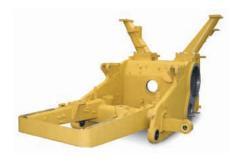
Frame and Castings. The D5N case and frames are built to absorb high impact shock loads and torsional forces.
