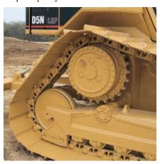
**Elevated Final Drive.** Final drives are isolated from ground and work tool induced impact loads for extended power train life.
